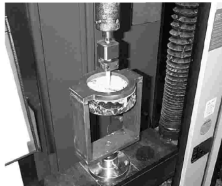
Figure 3 – A test setup for pullout testing.
